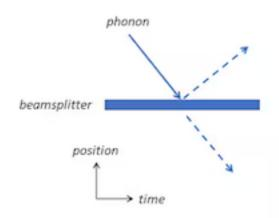
A beam splitter for phonons — the phonon enters a superposition state where it is both reflected and transmitted until it is detected. A.N. Cleland
